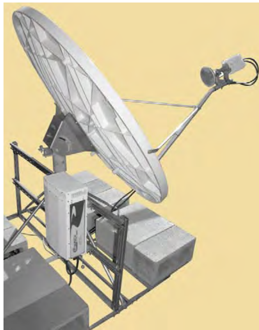
Figure 3-1. ODM-840 Temporary Field Installation Example
